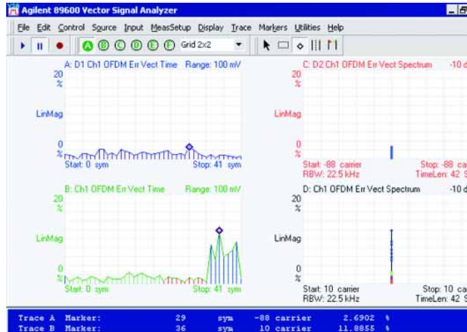
Figure 6-30 Error Vector Time and Error Vector Spectrum traces using a single WiMAX frequency subcarrier. The upper pair of traces shows the results for the pilot subcarrier at index = -88. The lower pair shows the results for a data subcarrier at index = 10 (example from Agilent 89600)
