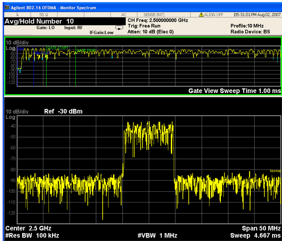
Figure 3-33 Monitor Spectrum Measurement - Gate View
